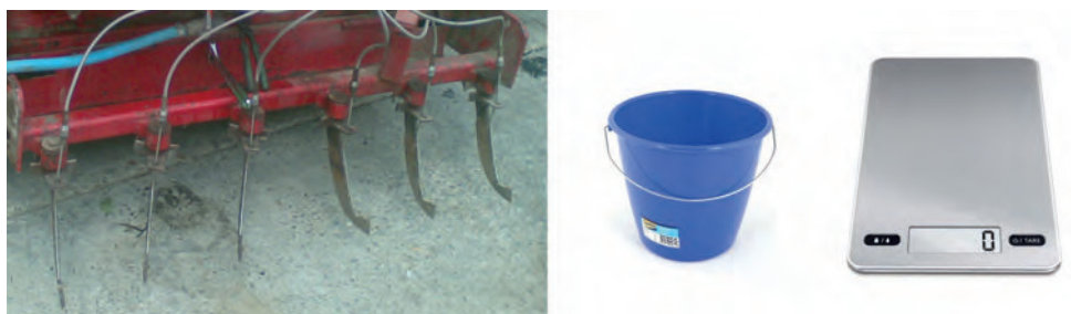
Fig. 4. Soil-disinfection machine injectors, pattern measurement.
