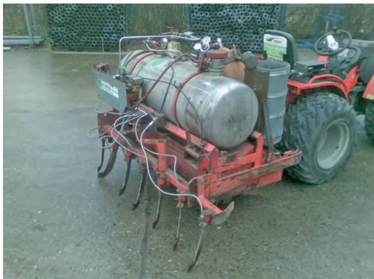
Fig. 2. Typical soil-disinfection machine.
