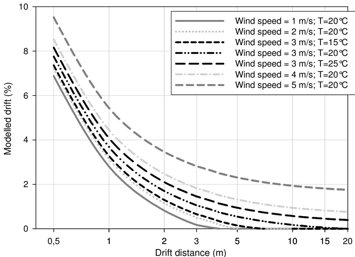
**Figure 4:** Drift curves for the reference spraying on a meadow under different climatological conditions
