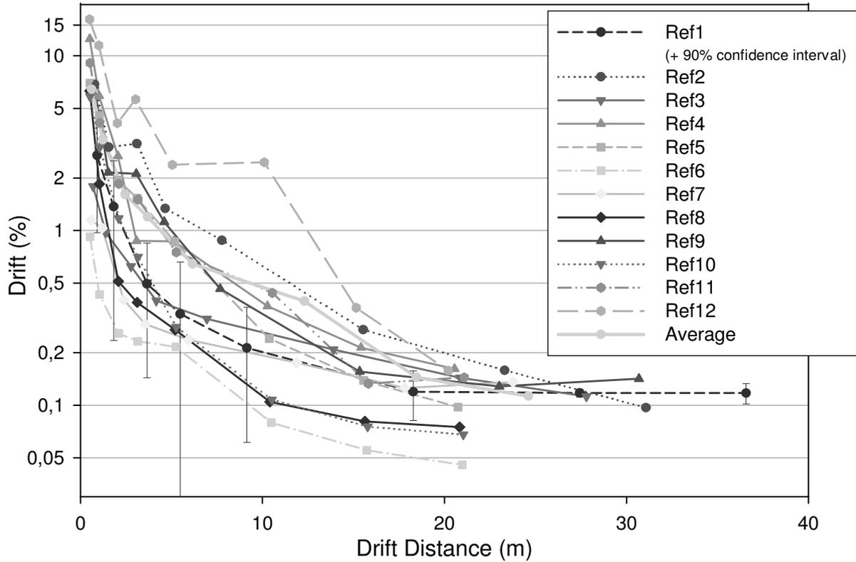
**Figure 3:** Drift data for the different reference sprays (+ average)
