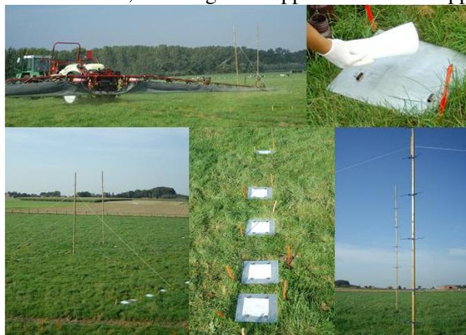
**Figure 1:** Some pictures of the experimental set-up for the field drift measurements
