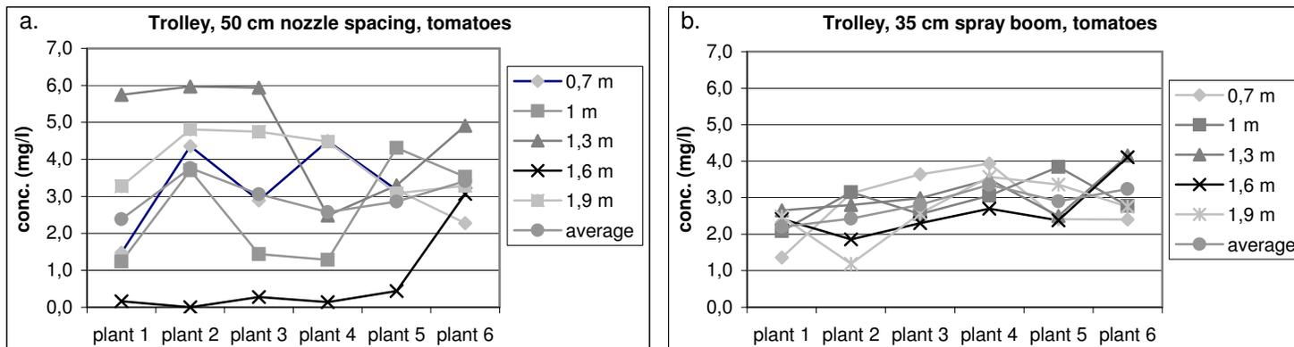
Fig. 5. Results of the deposition tests in the tomato crop with the trolley
