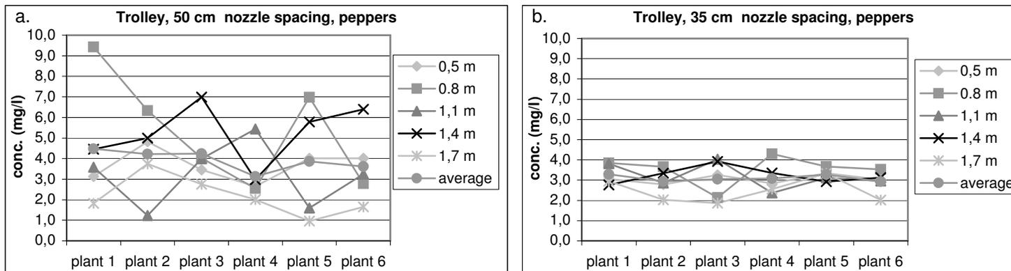
Fig. 3. Results of the deposition tests in the pepper crop with the trolley
