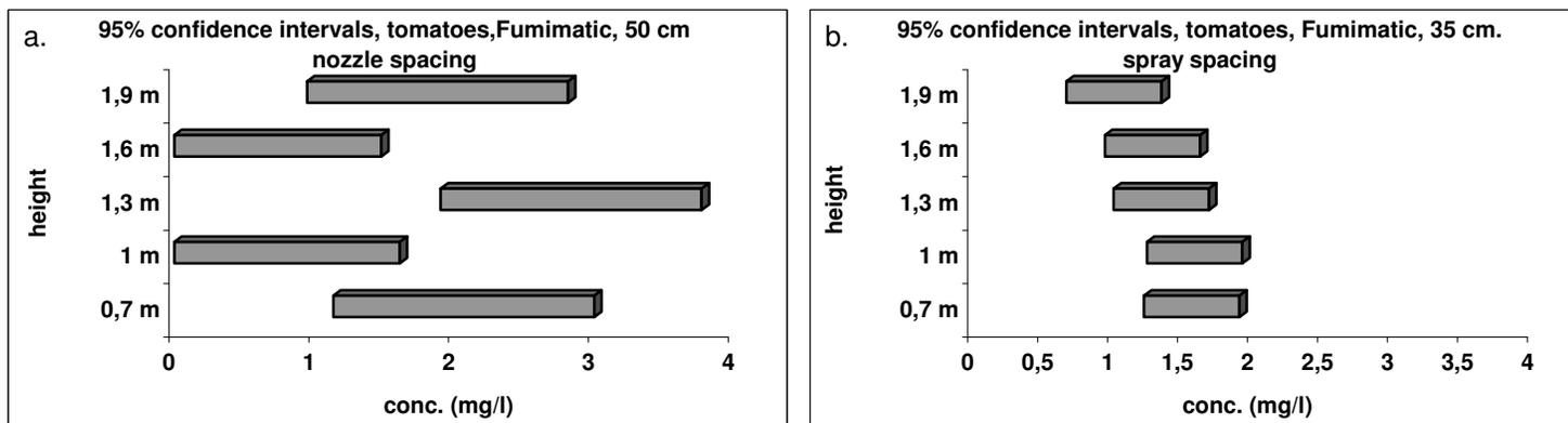
Fig. 6. 95% confidence intervals for the deposition on the topside of the leaves in tomatoes using the Fumimatic
