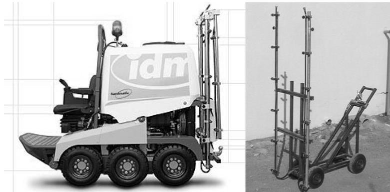
Fig. 1. The Fumimatic and the manually pulled trolley, both equipped with vertical spray booms
