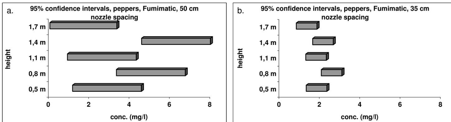
Fig. 4. 95% confidence intervals for the deposition on the topside of the leaves in peppers using the Fumimatic
